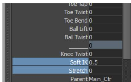
The stretch system works alongside the softIK, running the same math to determine at which point the stretch begins. The higher the softIK value, the sooner the stretch begins. Unlike a lot of stretch systems this means that the joints start stretching before they lock out.
